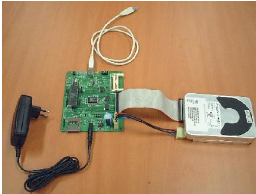
IDE hard disk setup for USB Mass Storage kit
